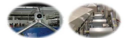
**COOLER** This small cooler has variable speed control that reduces substrate temperature thus making handling temperature operator friendly
